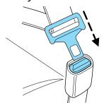
Grasp the shoulder portion and pull downward until the entire belt is pulled out.
